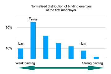
Figure 10: Representation of the binding energy distribution of the first monolayer of adsorbate.  $E_{10}$  (resp.  $E_{90}$ ) represents the binding energy after 10% (90%) of desorption.  $E_{mode}$  corresponds to the  $E_b$  of the largest number of adsorption sites.
