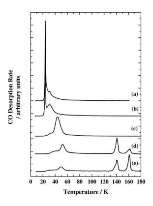
Figure 11: The effect of water on the desorption of CO ice. TPD of  $^{13}$ CO deposited at 8 K (a) on a gold substrate; (b) on low density amorphous water ice deposited at 120 K; (c) on low density amorphous water ice deposited at 70 K; (d) on high density amorphous water ice deposited at 8 K; and (e) deposited simultaneously with  $H_2O$  at 8 K. Heating rate = 0.08 K s<sup>-1</sup>. Traces are offset for clarity. Reproduced from Collings et al.  $^{164}$
