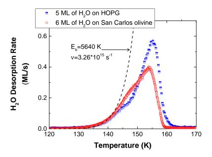
Figure 8: Comparison of TPDs of solid water from HOPG or San Carlos olivine surfaces. The dashed curve is an exponential trend obtained by using an  $E_b$ =5640 K and a  $\nu$ =3.26 ×  $10^{15} {\rm s}^{-1}$ .
