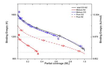
Figure 13: Binding energy distributions of pure CO and  $N_2$  (dashed lines) and of a 0.65 ML CO - 0.35 ML  $N_2$  mixture (solid lines) on c-ASW obtained using the classical inversion method. Reproduced from Nguyen et al.<sup>223</sup>
