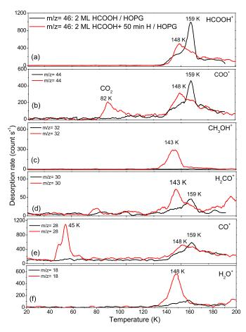
**Fig. 5.** TPD curves of HCOOH and HCOOH + H films on graphite (HOPG) surface for different masses. Black line: 2 ML of HCOOH ice on HOPG surface at 10 K; red line: 2 ML HCOOH + 50 min H atoms on HOPG surface at 10 K.
