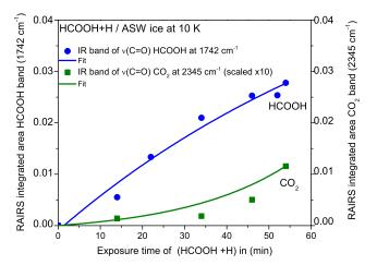
**Fig. 8.** Kinetic evolution of (HCOOH+H) system as a function of the exposure time (in s) of HCOOH and H beams on the ASW ice surface. The water ice film of 10 ML thickness is grown at 110 K, and cooled down to 10 K. The data are derived from the integrated areas below the RAIR absorption bands of HCOOH and CO<sub>2</sub> at 1729 cm<sup>-1</sup> and 2345 cm<sup>-1</sup>, respectively.
