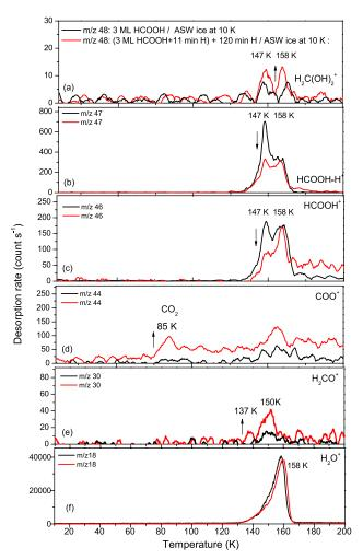
**Fig. 7.** TPD curves of HCOOH and HCOOH + H films on np-ASW ice surface for different masses from 10-200 K. Black line: 3 ML of HCOOH on 10 ML thickness of an ASW ice film prepared at 110 K and cooled down to 10 K, Red line: (3 ML HCOOH +11 min H) with an additional H atom bombardment of the film for 120 min on 10 ML thickness of an ASW ice film held at 10 K.
