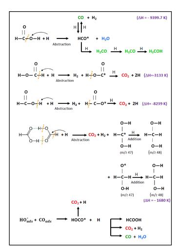
**Fig. 9.** Chemical reaction routes for the hydrogenation HCOOH+H reaction on cold graphite (HOPG) and ASW ice surfaces involving monomer and dimer of formic acid.
