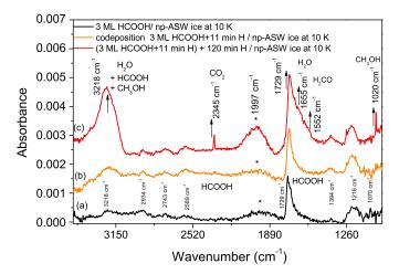
**Fig. 6.** RAIR spectra of HCOOH and HCOOH + H films on np-ASW of 10 ML thickness, deposited at 110 K and cooled down to 10 K. (a) 3 ML HCOOH on np-ASW ice surface at 10 K, (b) 3 ML HCOOH + 11 min H on np-ASW ice surface at 10 K, (c) (3 ML HCOOH + 11 min H) + 120 min H on np-ASW ice surface at 10 K.
