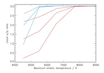
Figure 2.6: The H<sub>2</sub> ortho/para ratio as function of the maximum kinetic temperature reached in J-type shocks. Results are displayed for preshock densities of  $10^4$  cm<sup>-3</sup> (red) and  $10^5$  cm<sup>-3</sup> (blue) and for initial ortho/para ratios of 0.01, 1.0 and 2.0.
