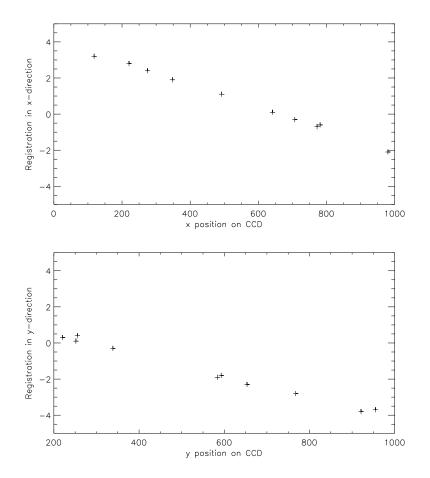
Figure 3.6: Registration in the CFHT data. The relative position of stars taken in the continuum filter (Br $\gamma$ , z=0.01) and v=1-0 S(1) filter as a function of absolute position in the v=1-0 S(1) filter for 10 stars.
