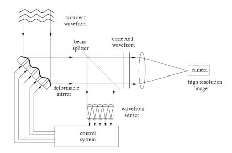
Figure 3.1: Schematic view of an adaptive optics system.
