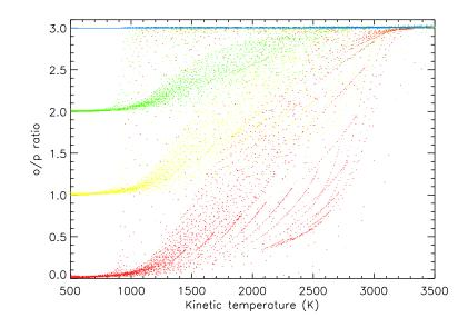
Figure 2.5: The  $H_2$  ortho/para ratio as function of the maximum kinetic temperature reached in C-type shocks. Each dot corresponds to a shock model. Red is for an initial ortho/para ratio of 3, green for 2, yellow for 1 and red for 0.01. The ortho/para ratio only changes between 800 and 3200 K.
