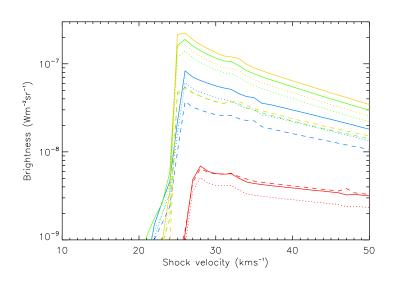
Figure 2.16: [FeII] emission in J-type shocks as a function of shock velocity. Brightness is shown for the transitions at 1.257  $\mu$ m (full line), 1.644  $\mu$ m (dotted line) and 17.936  $\mu$ m (dashed line). Brightness is displayed for four different preshock densities: 10<sup>4</sup> cm<sup>-3</sup> (red), 10<sup>5</sup> cm<sup>-3</sup> (blue), 10<sup>6</sup> cm<sup>-3</sup> (green) and 10<sup>7</sup> cm<sup>-3</sup> (yellow).
