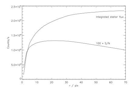
Figure 3.5: Aperture photometry of the calibration star HR1950. The total count rate within radius r is shown as well as the S/N ratio. The latter has been multiplied by 100. The S/N ratio peaks at a radius of ~23 pixels.
