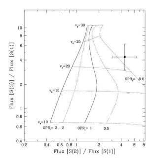
Figure 2.8: Diagnostic diagram of pure rotational  $H_2$ emission. Model predictions are shown for a C-type shock model with preshock density  $5 \times 10^5$  cm<sup>-3</sup> as a function of shock velocity and initial ortho/para ratio (OPR). Predictions are from (Timmermann 1998). Taken from Neufeld et al. (1998).
