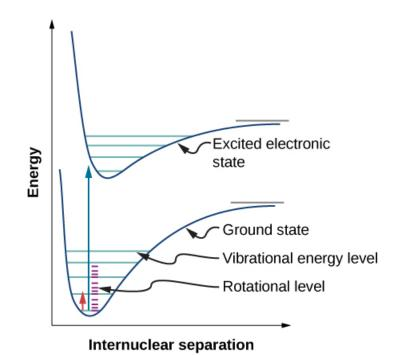
FIGURE 2.1: Representation of the Morse potential curve (blue curve), displaying the different energy levels. Two Morse potential curves correspond to different electronic levels, here the ground state and excited state. Within each electronic state, the different vibrational and rotational levels are shown. Credit: Ling *et al.* (2016)
