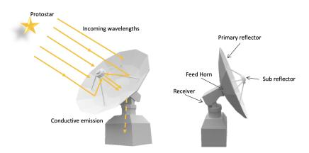
FIGURE 2.3: Schematic overview of the single-dish antenna- Cassegrain system
