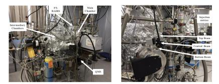
FIGURE 2.6: VENUS apparatus. *left:* front view of VENUS, displaying the intermediary chambers, main chamber, FT-RAIRS and QMS. *right:* Side view of VENUS showing the different three molecular injection entries (i.e., top, central and bottom beams) (atomic hydrogen entry not included).
