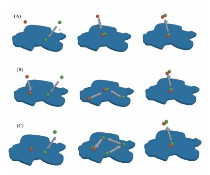
FIGURE 1.10: Surface Chemistry of species X and Y on dust grain (g) (a) Eley-Rideal mechanism (b) Langmuir-Hinshelwood mechanism (c) Kasemo-Harris mechanism.
